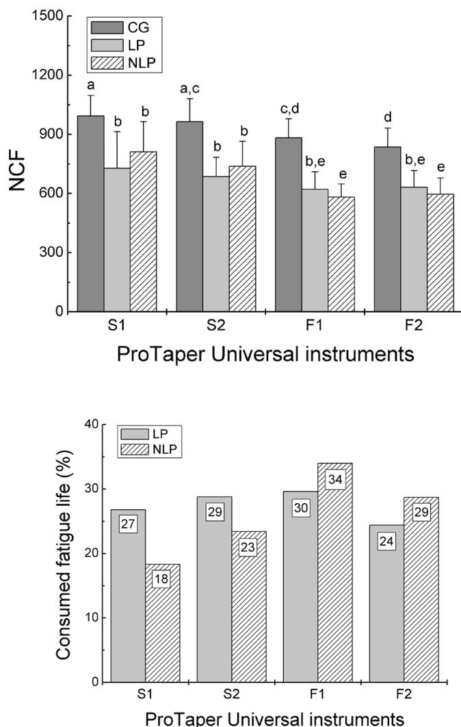
**Figure 2** - (a) Mean values of the number of cycles to failure (NCF) in the fatigue-tested new and used instruments. Differently labeled columns represent statistically significant differences ( $p = 0.05$ ); (b) Mean values of consumed fatigue life in the fatigue-tested used instruments.
