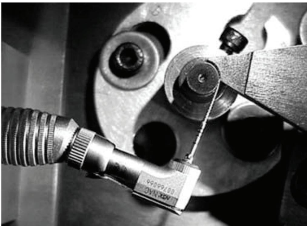
Figure 1 - Artificial canal with an instrument attached
