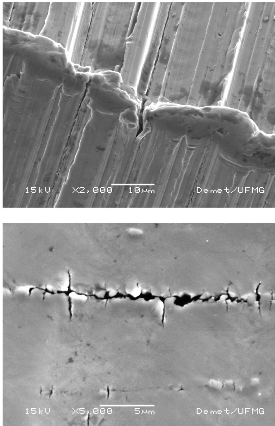
**Figure 3** - Scanning electron microscopy images of (a) the surface of a F1 PTU instruments used for the shaping of 5 molars in the group with lateral pressure motion showing transversal cracks at 2.8 mm from the tip; (b) the surface of a F1 ProTaper Universal instrument (PTU) used for the shaping of 5 molars in the group without lateral pressure motion, showing a longitudinal crack at the same tip level.
