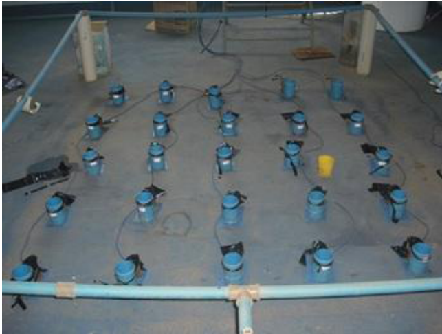
Figure 3 – Test device in the laboratory with the catch cans
