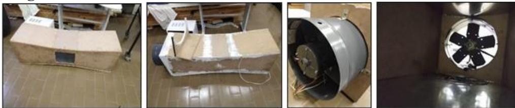
Figure 6 - Mounted structure of the tunnel and details of the installed exhaust.
