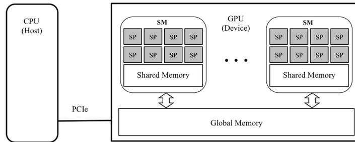
Fig. 2. Overview of a GPU architecture
