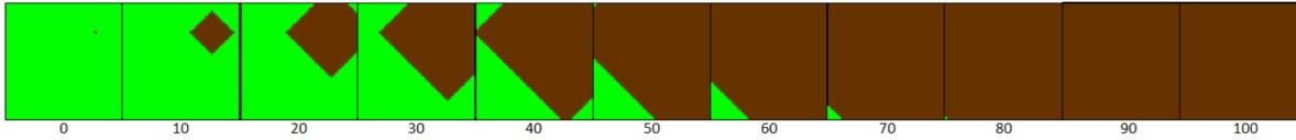
Fig. 4. Heat spread over the cellular space. Green (inert), Brown (Burning).
