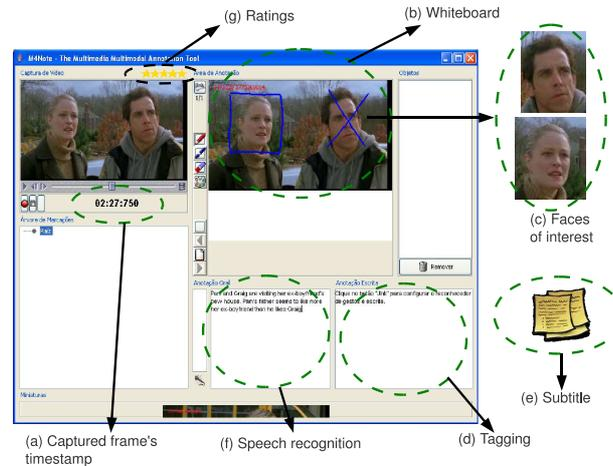
Fig. 2. Peer-level enrichment environment using the M4Note application. Dashed ellipses represent extracted metadata that describes user's preferences.
