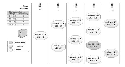
Fig. 1. Sensor field and a storage assignment (SA)
