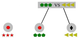
(b) Tree obtained after the first merge performed by the aggregattion scheme (Step 3). Leaves are represented by circles with the symbol of the corresponding class inside, and the labeled objects are presented in each leaf according to the cluster they were assigned to. Each internal node is represented by a rectangle with the definition of the binary sub-problem that it addresses.
