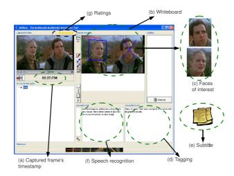
Fig. 2. Peer-level enrichment environment using the M4Note application. Dashed ellipses represent extracted metadata that describes user's preferences.
