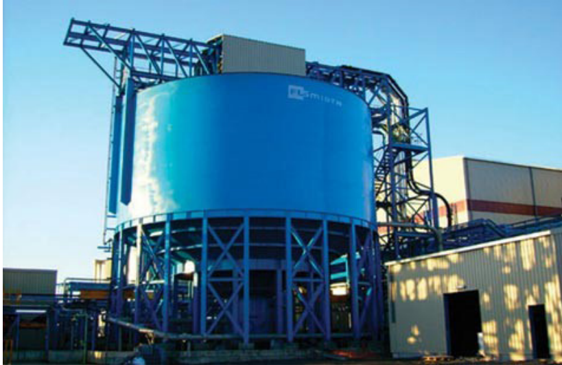
Figura 8 – Deep Cone Paste Thickeners/EIMCO
